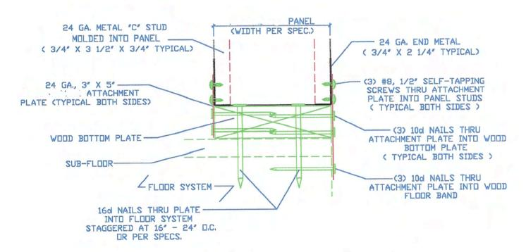
( WITH WOOD PLATE NAILED DOWN AND ATTACHMENT PLATES TO FLOOR SYSTEM )
