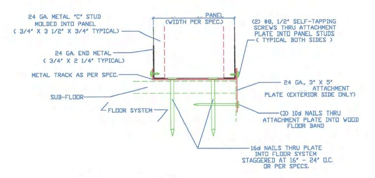
( WITH METAL TRACK NAILED DOWN AND ATTACHMENT PLATES TO FLOOR SYSTEM)
