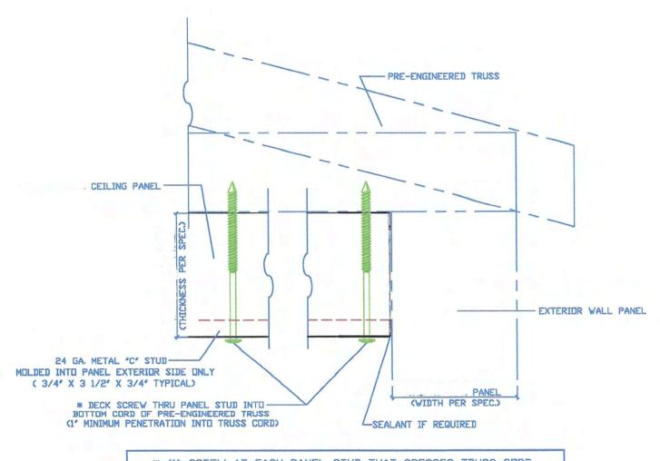
\* (1) SCREW AT EACH PANEL STUD THAT CROSSES TRUSS CORD (1" MIN. PENETRATION WITH DECK SCREW INTO TRUSS CORD)
